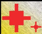
A pair of Box Cross Test Structures for the Measurement of CMP Dishing
