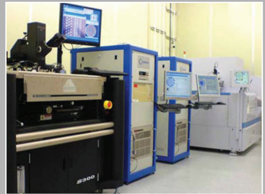
Centaur integrates with both TSK UF3000 12"inch Auto prober and Cascade S300 12"inch Semi Auto Prober
